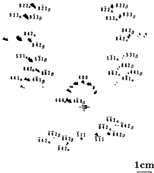
FIGURE 2 Indexed Laue pattern recorded at 120K from the same p -terphenyl single crystal. Again the cross indicates the direct beam position. This pattern consists of a superposition of patterns from the \alpha and \beta low temperature phases.
